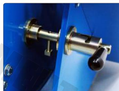
Drum Position Lock with Safety Switch
